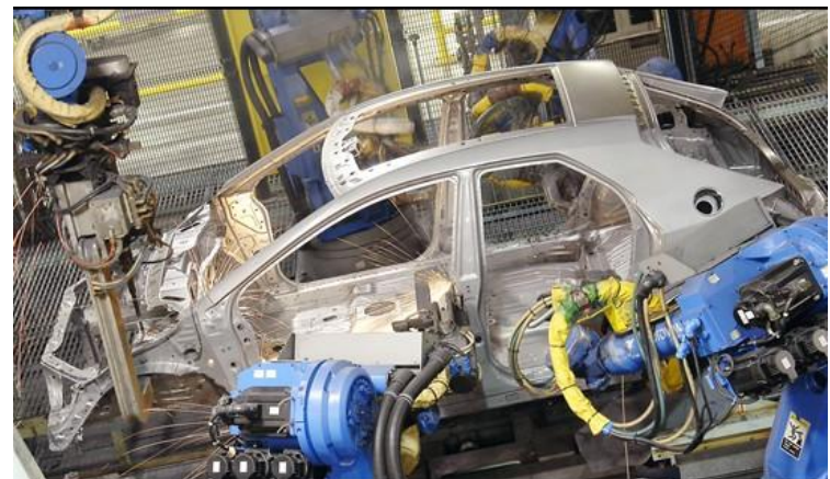
Honda of the UK Manufacturing Ltd Weld - Spot Robot Line
